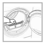
Removing the filter: 1. Pull the plastic grip of the filter upwards (*see diagram*).
